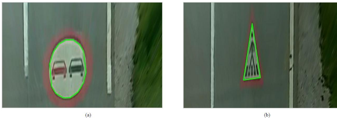
Fig. 4. Detection of different shapes. (a) Circular, prohibitory sign (No overtaking). (b) Triangular, warning sign (Pedestrian crossing)
